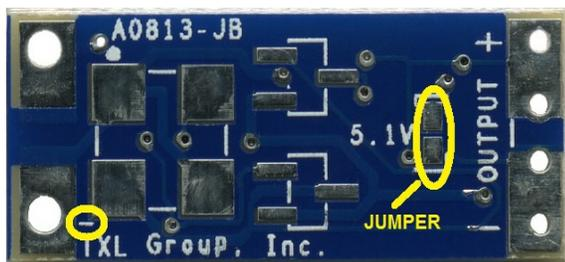
Figure 3 – Jumper Placement on the Backside of the Board to Select 5.1 Volt Regulation
